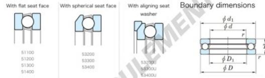
Thrust Ball Bearings - Single Direction
